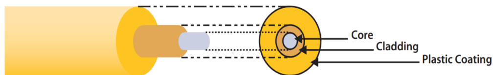
Fig 1.1 : The composition of optical fiber [1].
