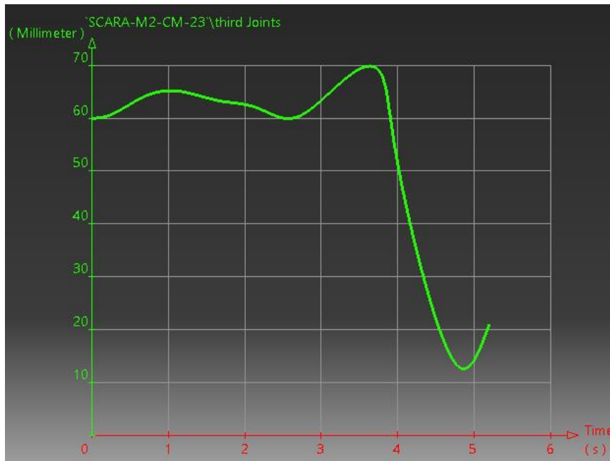
Figure IV. 22 Third joint position with CATIA V5
