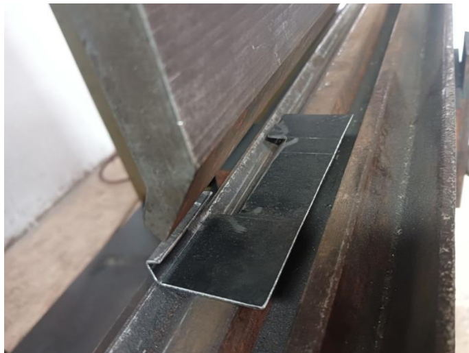
Figure IV.4: Manufacturing step in the Hydraulic Sheet Metal Bending Machine
