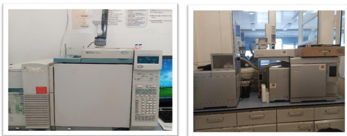
Figure IV 4: Le montage GC/ MS.
