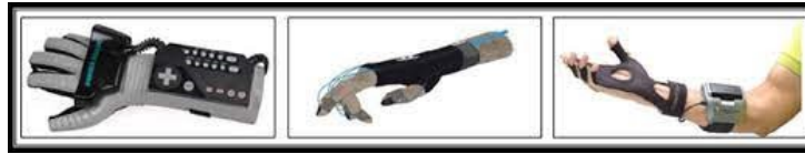
FIG. 1.6 : Several types of smart gloves : Power Glove (left), DT-Data Glove (Center), Cyber Glove (right)
