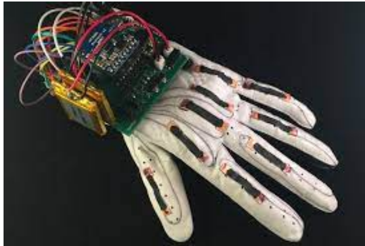
FIG. 4.6 : SL Glove Implementation
