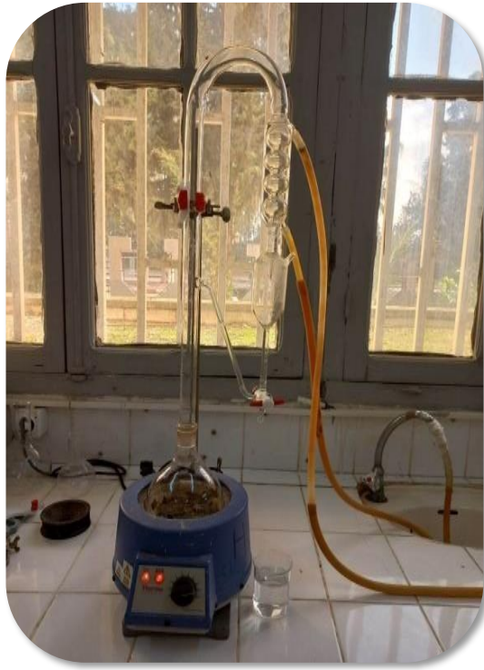
Figure 12 : Montage hydro distillation de type CLEVANGER (Photo originale, 2024).
