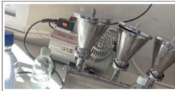
Figure 29: rompe de filtration
