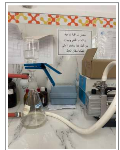
Figure 18: rampe de filtration + pompe a vide (Photo originale, 2024)
