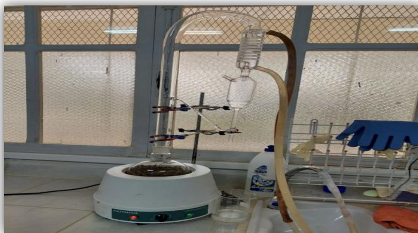
Figure 9: hydrodistillation (type Clevenger) (originale)
