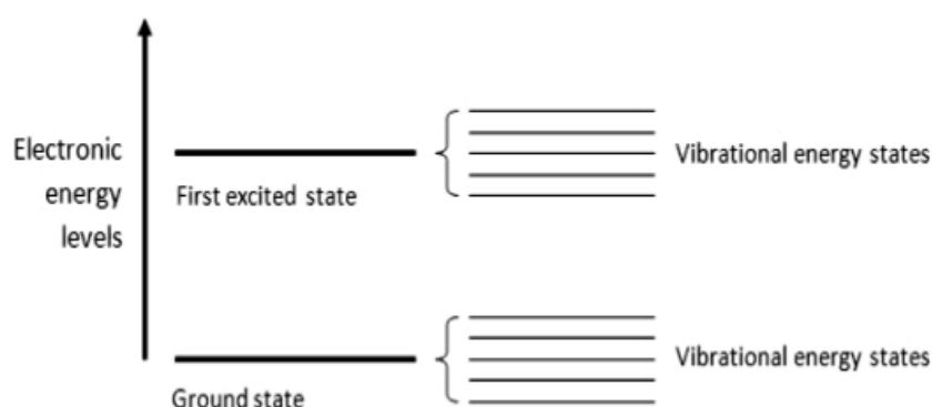
Fig.X.11 A schematic representation of the quantized electronic and vibrational energy levels of a molecule: to raise the electronic energy state of a molecule from the ground state to the excited state will cost more energy than to raise the vibrational energy state.
