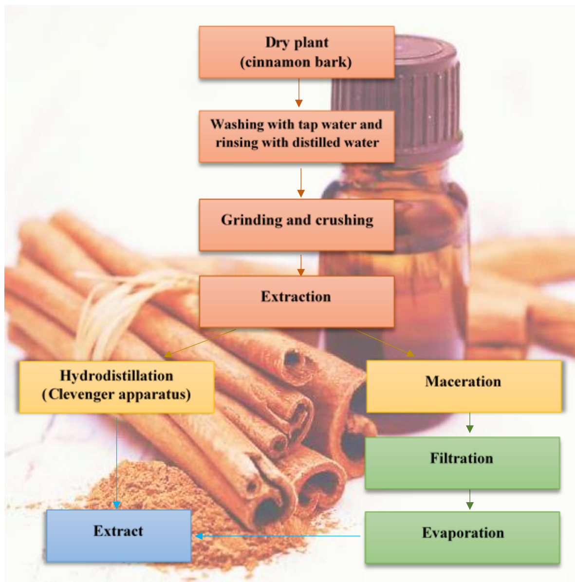
Figure 4.7. Flowchart representing the two extraction methods using
