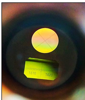
Figure 5.5. Refractive index as shown on refractometer
