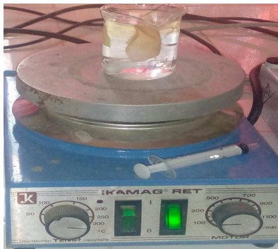
Figure IV.7: peace of membrane during the release in the Phosphate Buffer Saline.
