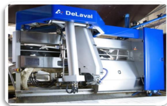
Figure 5: Robot de traite de Delaval. [53]
