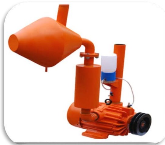
Figure 18: Pompe à vide. [27]
