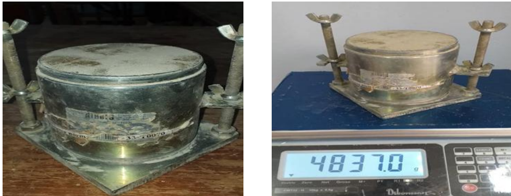
Figure 3.10: compactage du sol.
