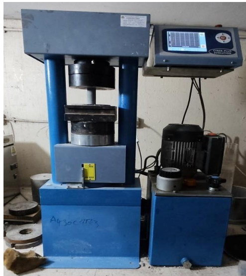
Figure IV.17. La presse de compression simple.
