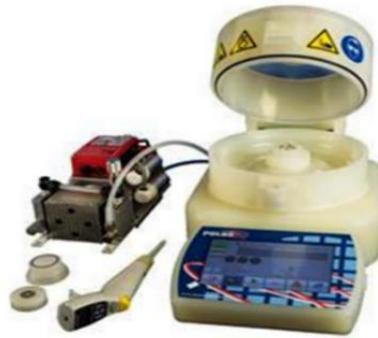
Figure 3.8 : VTC100C2 SPIN COATER
