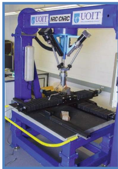
**Figure 1. 5** robot parallèle a 3ddl[25]
