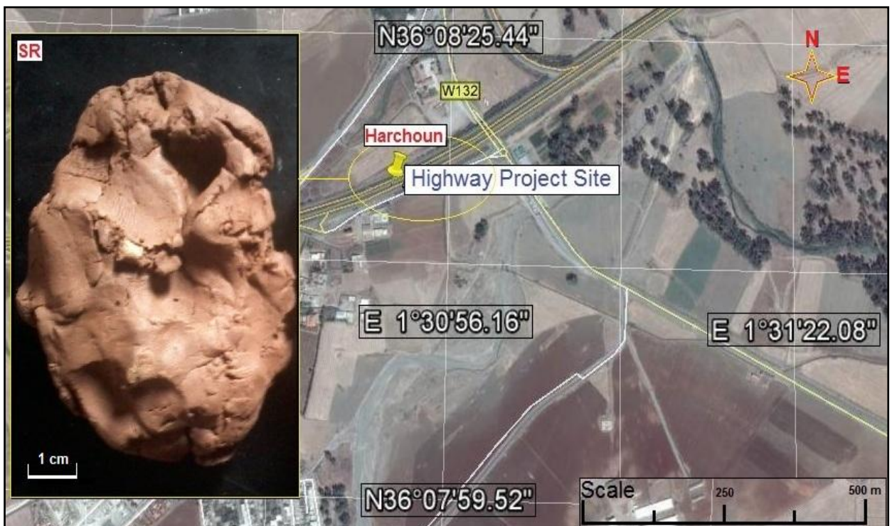
Figure 4.1. Sampling of red clay soil from a depth of 5m in the region of Harchoun, Algeria.
