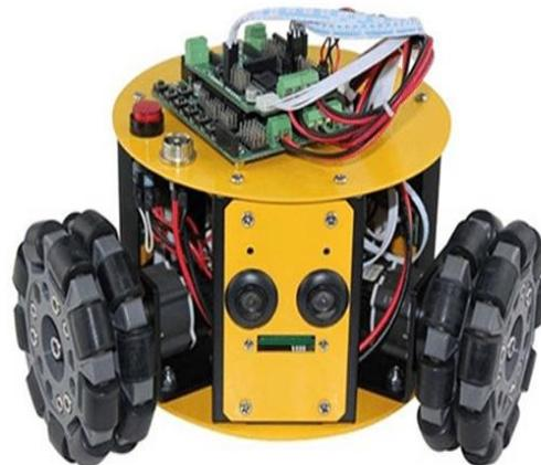
Figure I.16 : Robot omnidirectionnel
