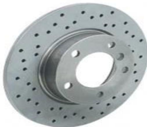
**Figure I.11** :disque percé [7]
