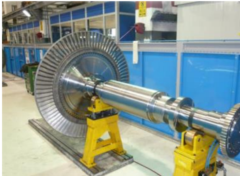
Figure II-26 : Rotor Turbine BP
