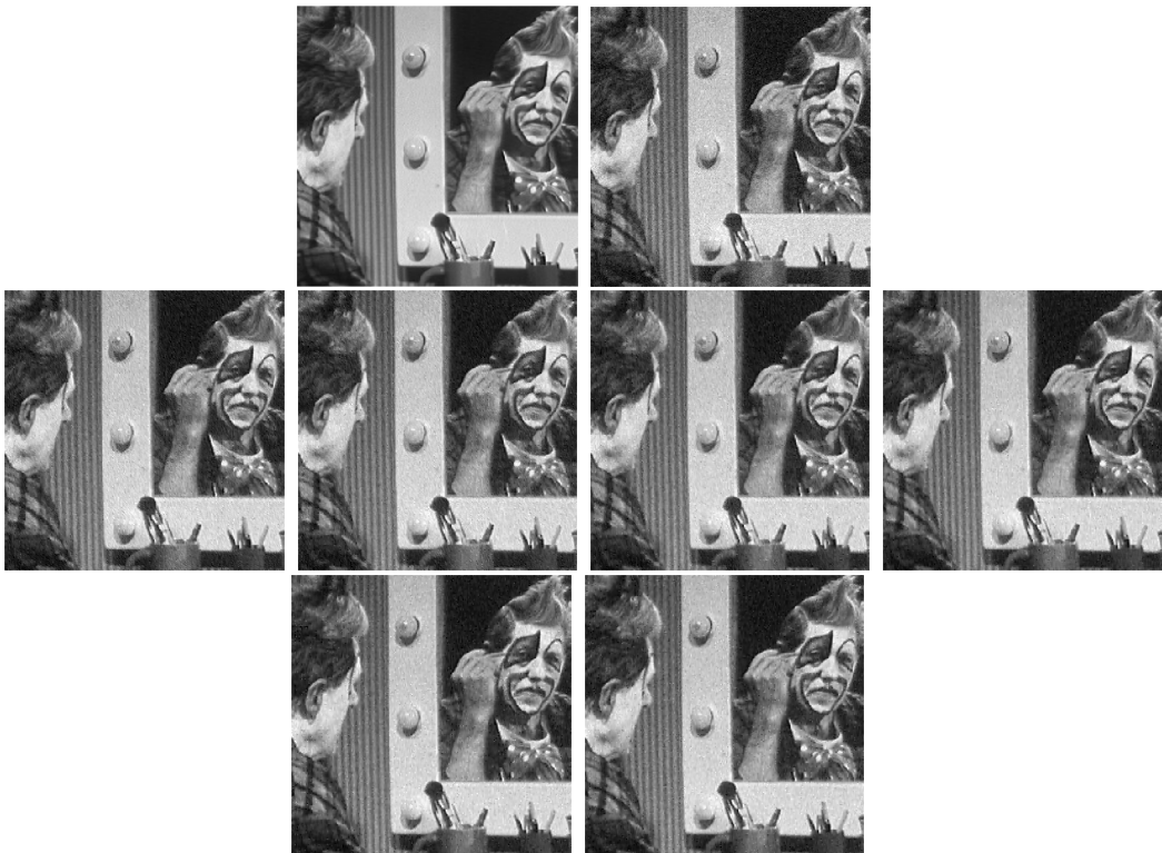
Figure 3.4: From left to right and from top to bottom : Original image. Noised image with ( \sigma = 0.002 ). First line : Denoised image with \alpha = 1 , \alpha = 1.2 , \alpha = 1.4 , \alpha = 1.6 . Second line : \alpha = 1.8 , \alpha = 2 .
