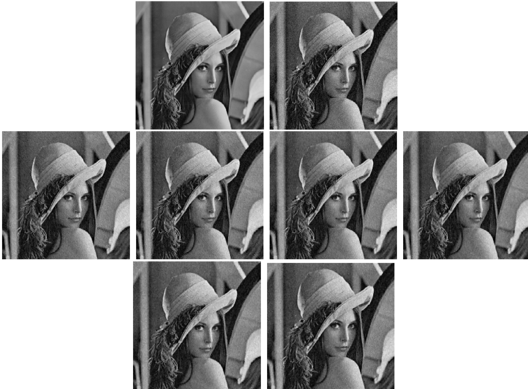
Figure 3.2: From left to right and from top to bottom : Original image. Noised image with ( \sigma = 0.002 ). First line : Denoised image with \alpha = 1 , \alpha = 1.2 , \alpha = 1.4 , \alpha = 1.6 . Second line : \alpha = 1.8 , \alpha = 2 .
