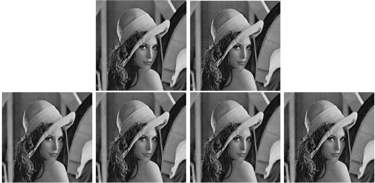
Figure 3.6: From left to right and from top to bottom : Original image. Noised image with ( \sigma = 0.001 ). First line : Denoised image \alpha = 1 with k = 50 , k = 20 , and \alpha = 1.5 with the same values of k .
