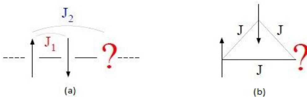
Fig 3.2: (a): Frustration due to the competition between several couplings, J_1 > 0 et J_2 > 0 . (b): Frustration géométrique, J > 0 .
