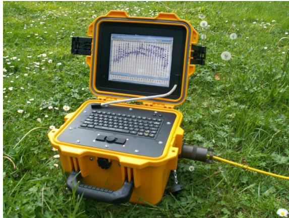
Figure.3.2: Le seismographe SUMMIT X STREAM Pro.
