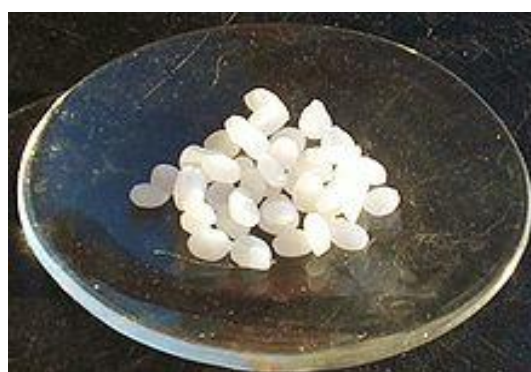
Figure A.6: Hydroxyde de sodium (NaOH).
