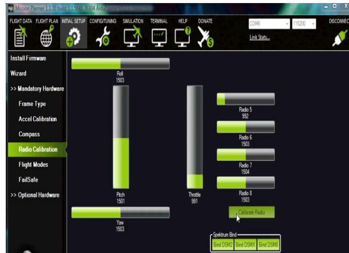
FIGURE 4.21 – Calibration de la radio-commande
