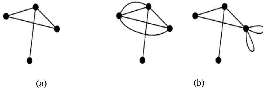
Figure II-8 : (a) Simple Graph, (b) non simple graph having multiple edge (left) non simple graph having loops(right).
