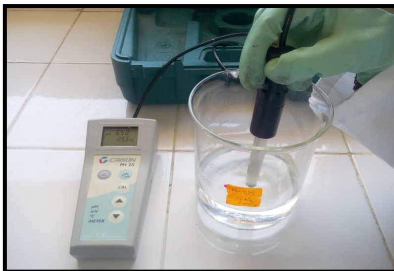
Figure 11: Mesure de pH de tampon phosphate (solution de conservation).
