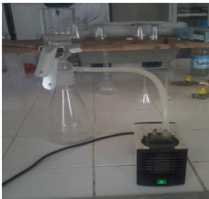
Figure IV.6: la rampe de filtration
