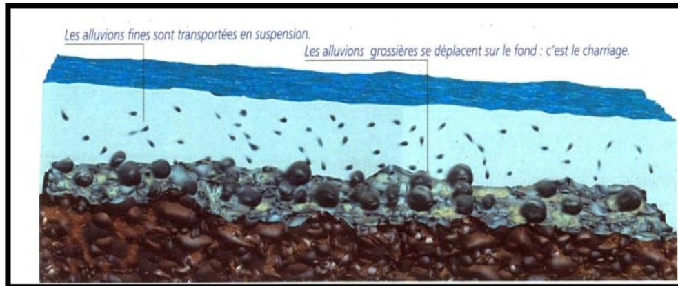
**Figure 8:** Mode de transport solide (SOGREAH, 2003)
